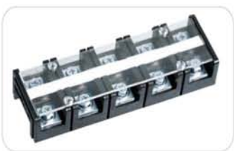
TC-1005 导线截面 wire section: 22mm 2 额定电流/电压 rated current/voltage: 100A/600V 长/宽/高 length/wide/high: 173.5/55/38mm
