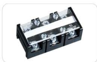
TC-603 导线截面 wire section: 14mm 2 额定电流/电压 rated current/voltage: 60A/600V 长/宽/高 length/wide/high: 83.5/41.2/32.5mm
