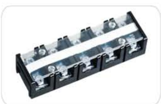
TC-605 导线截面 wire section: 14mm 2 额定电流/电压 rated current/voltage: 60A/600V 长/宽/高 length/wide/high: 145/43.2/32mm
