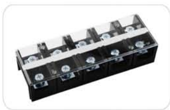
TC-1505 导线截面 wire section: 60mm 2 额定电流/电压 rated current/voltage: 150A/600V 长/宽/高 length/wide/high: 193/66/40.5mm
