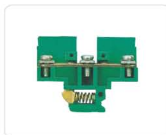
JH 10 15-60L 导线截面wire section: 0.75-2.5mm 2 额定电流/电压rated current/voltage: 24A/500V 厚/宽/高thick/wide/high: 54/65/10mm
