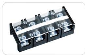
TC-1504 导线截面 wire section: 60mm 2 额定电流/电压 rated current/voltage: 150A/600V 长/宽/高 length/wide/high: 153.5/66/40.8mm
