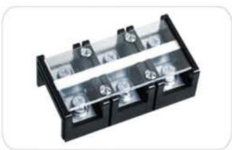
TC-2003 导线截面 wire section: 100mm 2 额定电流/电压 rated current/voltage: 200A/600V 长/宽/高 length/wide/high: 133/71/47.5mm
