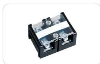
TC-602 导线截面 wire section: 14mm 2 额定电流/电压 rated current/voltage: 60A/600V 长/宽/高 length/wide/high: 58/42.5/35mm
