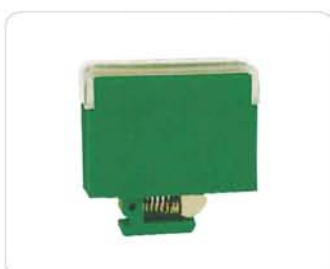
JF5-2.5/S2 导线截面wire section: 0.5-2.5mm 2 额定电流/电压rated current/voltage: 24A/660V 厚/宽/高thick/wide/high: 26/42/47mm
