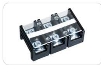
TC-1503 导线截面 wire section: 60mm 2 额定电流/电压 rated current/voltage: 150A/600V 长/宽/高 length/wide/high: 114.5/65.3/40.8mm
