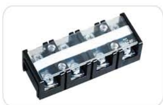
TC-604 导线截面 wire section: 14mm 2 额定电流/电压 rated current/voltage: 60A/600V 长/宽/高 length/wide/high: 111.2/41.2/32.5mm
